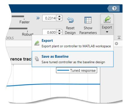
When you do so, the current **Tuned response** becomes the **Baseline response**. Further adjustment of the current design creates a new **Tuned response** line.
