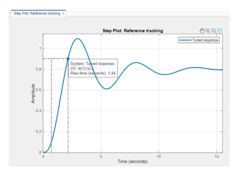
Moving the **Response time** slider far enough to meet the rise time requirement of less than 1.5 s results in more oscillation. Additionally, the parameters display shows that the new response has an unacceptably long settling time.
