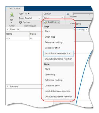
For example, to observe the closed-loop step response to disturbance at the plant input, in the **Step** section of the **Add Plot** menu, select Input disturbance rejection. The disturbance rejection response appears in a new figure.
