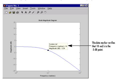
The following figure shows the Bode magnitude of the shaping filter.
