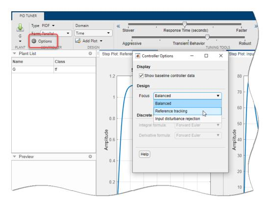
**PID Tuner** automatically retunes the controller coefficients with a focus on reference-tracking performance.
