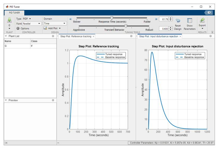
As in the PI case, the initial PIDF design balances reference tracking and disturbance rejection. Also as in the PI case, the controller yields some overshoot in the reference-tracking response, and suppresses the input disturbance with a similar settling time.
