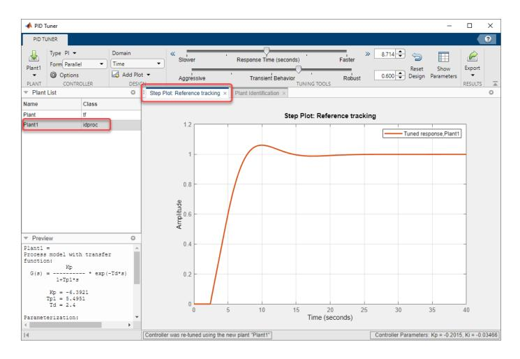
Tip To examine variables stored in the PID Tuner workspace, view the Plant List.
