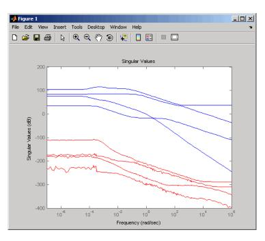
The reduction error is small compared to the original system so the reduced order model provides a good approximation of the original model.
